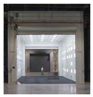
The booth incorporates re-circulation technology and uses filters complying with EPA NESHAP filtration requirements. Filters are located in the basement of the booths via a below-grate stairway.
