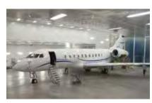
Air in a crossdraft booth flows from end to end, matching the natural flow of air across the aircraft. This provides excellent quality finishes. Making up about 75% of all aircraft paint booths, crossdraft booths are the most common style for aviation finishing operations.
