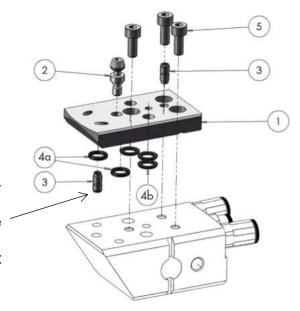
Removable location Pin – Can be removed so Intermediate Plate can be fitted to existing Special machine adaptors without modification.
